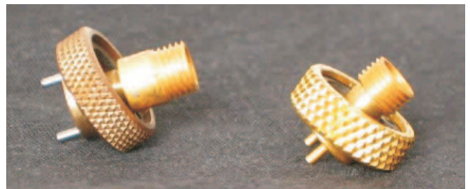
Fig. 6. Waveguide transitions with fixed (right) and demountable (left) horn
